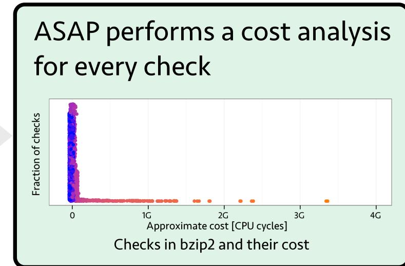
ASAP selects checks that maximize security for the desired overhead level. overhead: 9.2% security: > 90% Result of optimizing bzip2 with ASAP
