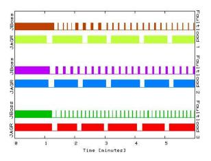
Figure 3. The client-perceived instantaneous availability of JBoss/PetStore and JAGR/PetStore under three different faultloads. Faults are injected every minute; JAGR manages to successfully and autonomously recover PetStore every time.
