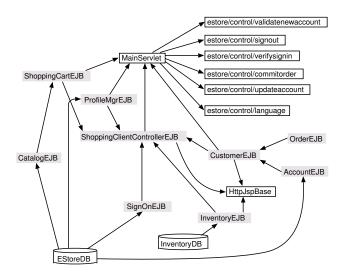
Figure 2. The AFPI-generated failure propagation map for PetStore 1.1. This is more complete and accurate than a map obtained based on the application's deployment descriptors. The boxes in the diagram are EJBs, Java Server Pages (JSPs), and/or servlets. Two databases are used, and are shown at the bottom.
