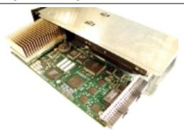
**Figure 8. A ROC-1 brick.** Each brick contains a 266 MHz mobile Pentium II processor, an 18 GB SCSI disk, 256 MB of ECC DRAM, four redundant 100 Mb/s network interfaces connected to a system-wide Ethernet, and an 18 MHz Motorola MC68376-based diagnostic processor. Eight bricks fit into a tray, and eight trays form the cluster, plus redundant network switches. See [Opp02] for more details.
